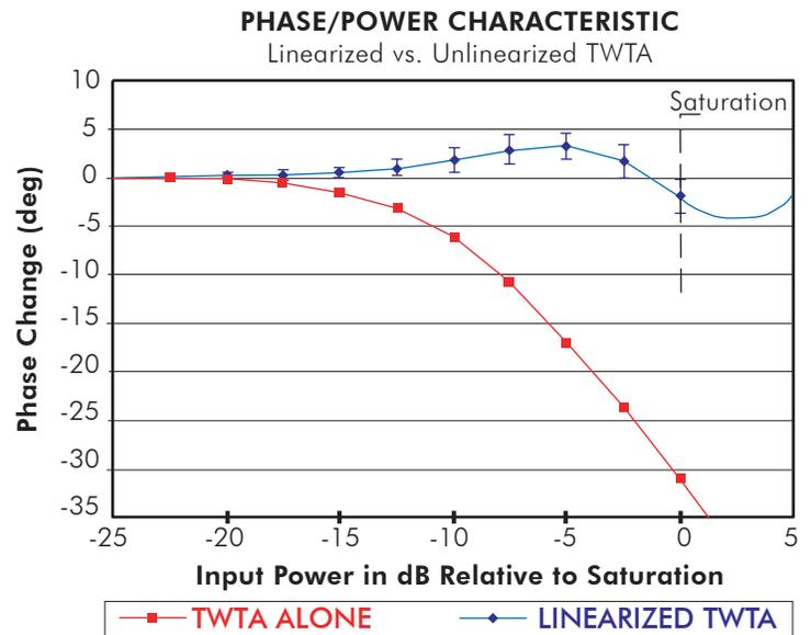
**FIGURES 3A & B : The Combination of a BAFL or WAFL type linearizer provides improved C/I and Near Constant Phase Transfer Characteristics. (Standard deviations shown represent a statistical sample of 38 units at center band and at band edges.)**
