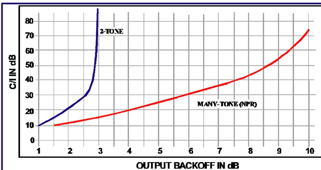
▲ Figure 10: C/I of an ideal linearizer for 2 and an infinite number of carriers (NPR)
