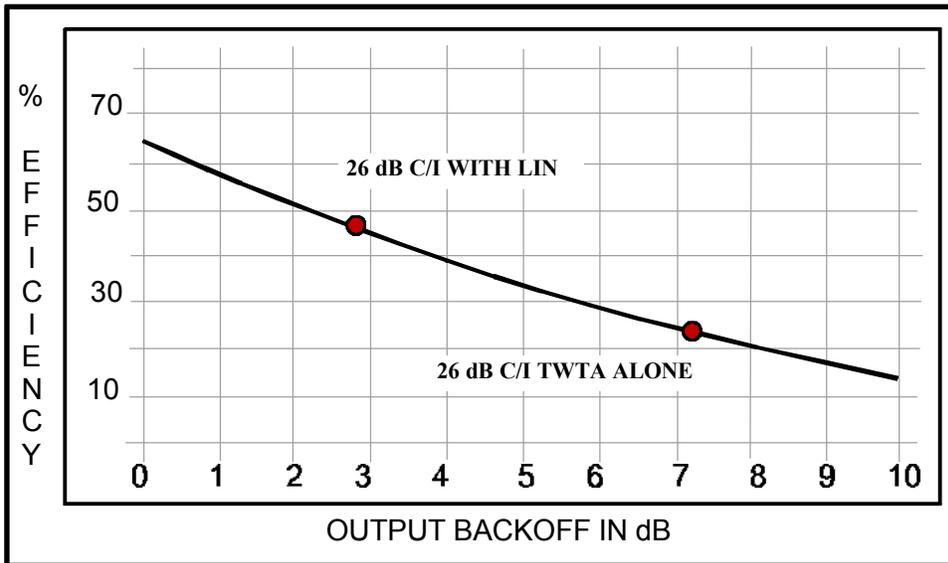
▲ Figure 19. A very significant increase in TWTA efficiency can be achieved for a C/I of 26 dB
