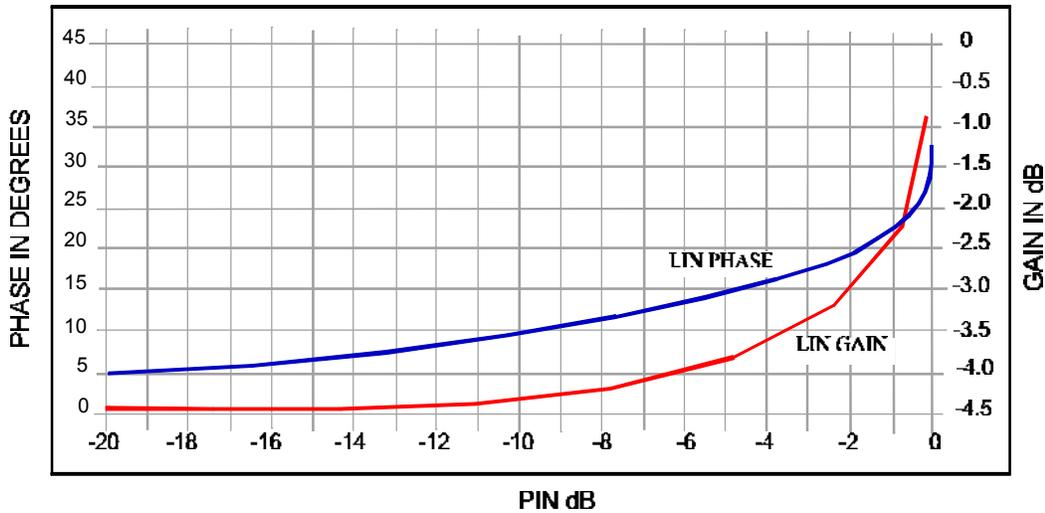
▲ Figure 9: An ideal PD linearizer response requires the gain and phase slope to become infinite as SAT is approached
