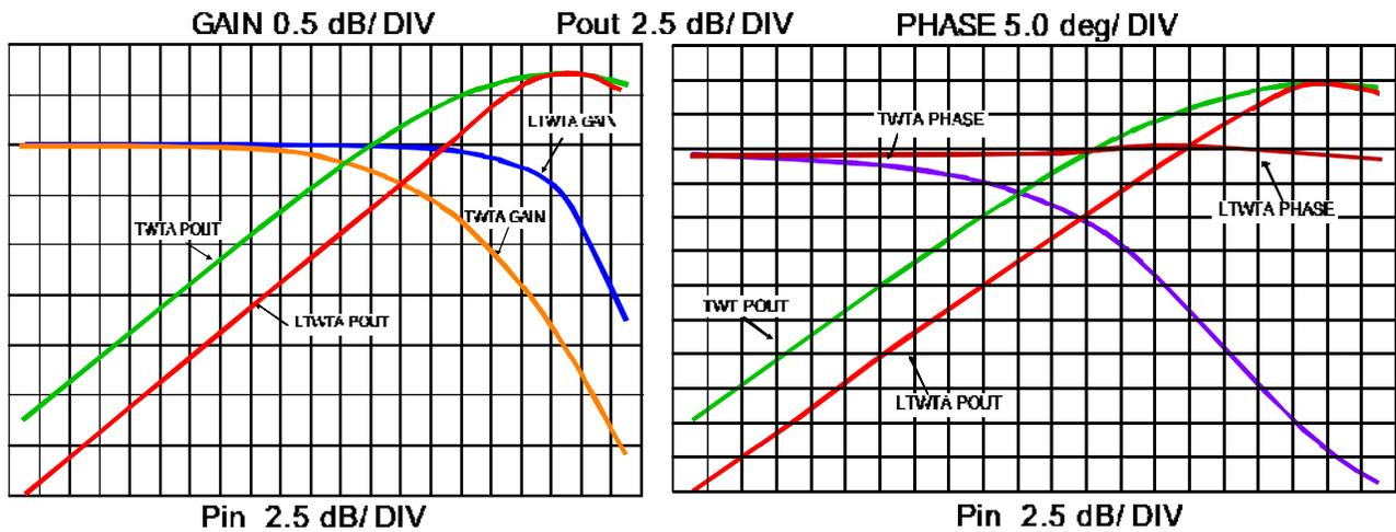
▲ Figure 13: Transfer characteristics of TWTA and linearized TWTA
