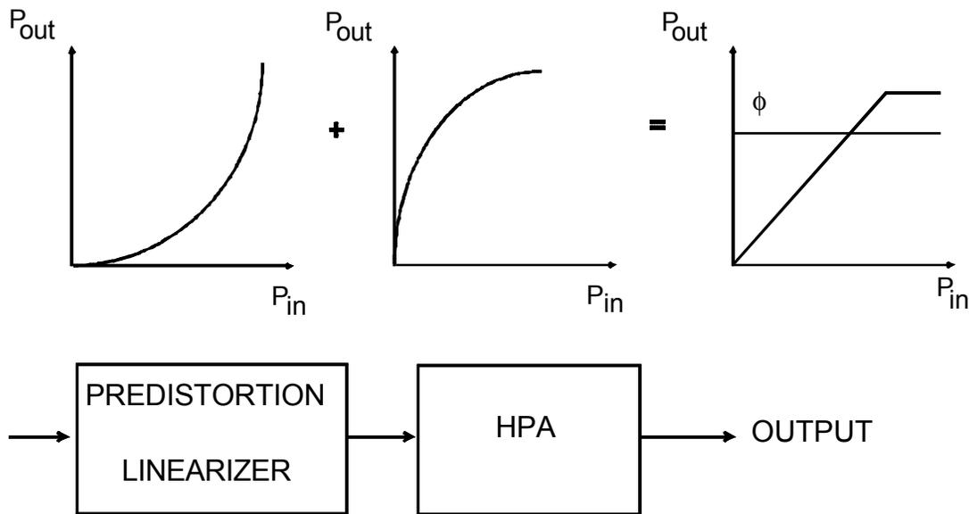
linearizer response needed to correct a given amplifiers transfer response. Figure 9 shows the response needed to ideally correct a typical TWTA. As SAT is approached the rate of gain and phase change become infinite.
