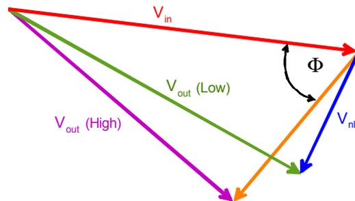
▲ Figure 11: Gain expansion can be produced by subtracting a linear path from a non-linear path
