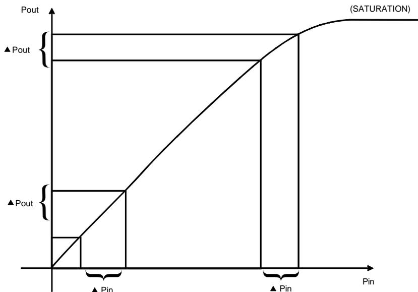
Figure 2. As an amplifier is driven closer to saturation, its output level will increase by a smaller amount, for a fixed increase in input signal.
