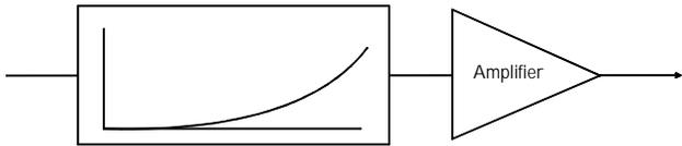
Figure 3c. Predistortion is relatively simple to implement, can provide wide bandwidth and is widely used with TWTA's.
