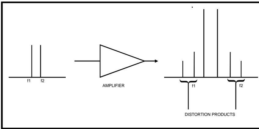
Figure 1. When two or more signals are amplified, distortion products appear in the vicinity of the desired signals.
