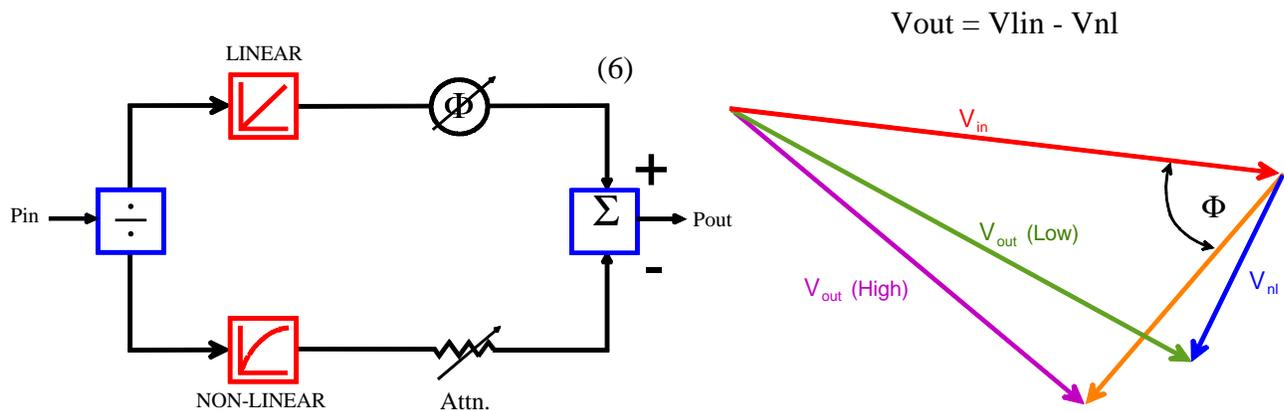
Figure 5. Gain expansion can be produced by subtracting a linear path from a nonlinear path.
