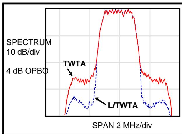
regrowth achieved by linearization as a function of OPBO. If a 2-tone  $C/I > 25$  dB can be achieved, the spectral regrowth will be  $> 30$  dB down. Linearization also improves the bit-error-rate (BER) of digital modulated signals. In general the greater the required BER, the greater the improvement provided by linearization.
