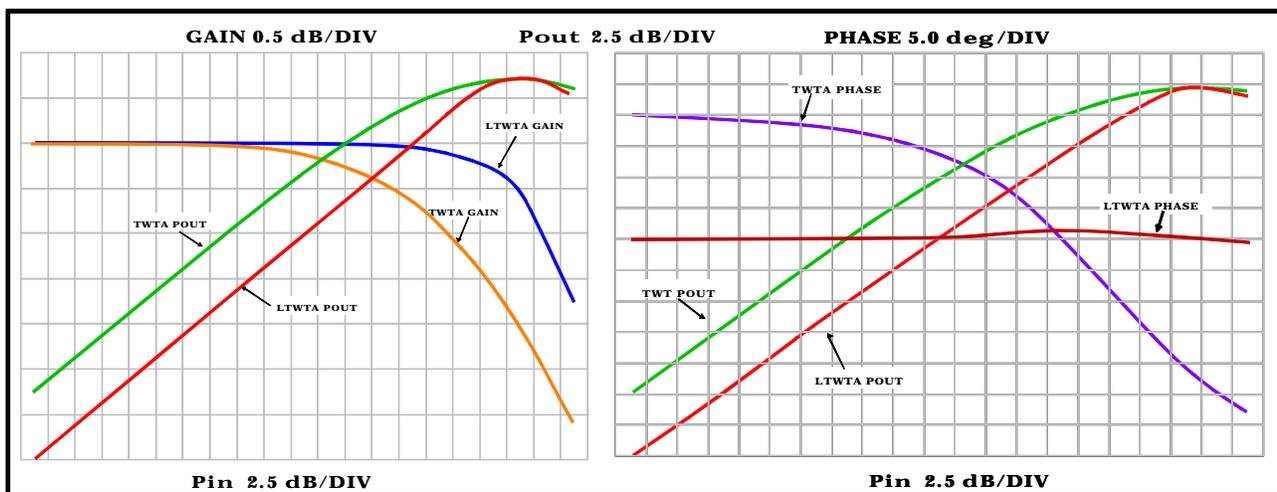
Figure 6. Transfer characteristics of TWTA and linearized TWTA.
