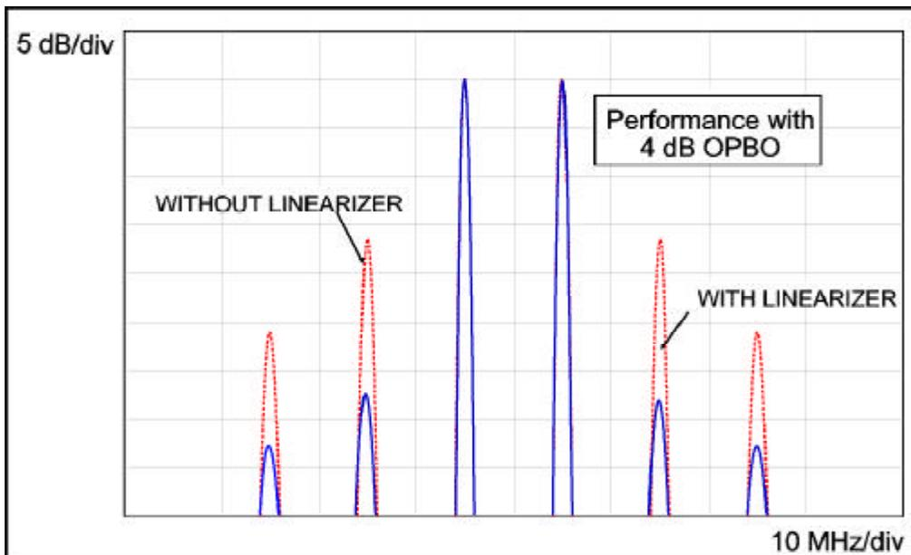
Figure 9. A two-tone C/I improvement of greater than 15 is common at 4 dB OPBO.
