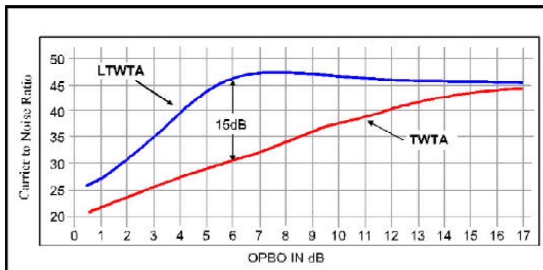
Figure 15. Reduction in spectral regrowth provided by linearization of a TWTA.
