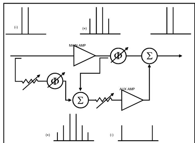
Figure 3a. Feedforward is relatively complex, but can provide wide-band and excellent distortion reduction.
