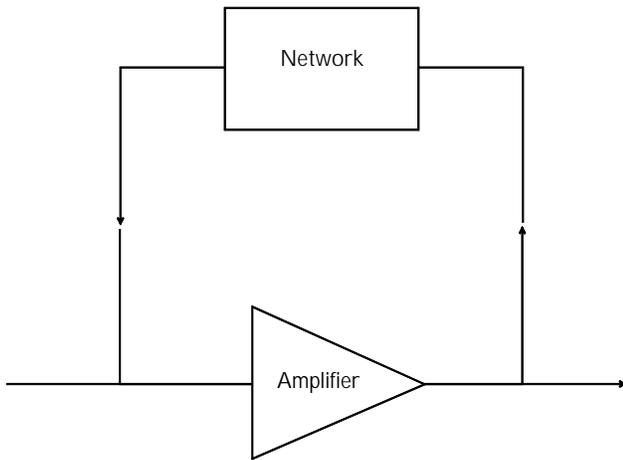
Figure 3b. Feedback is relatively narrow band and has potential stability problems.
