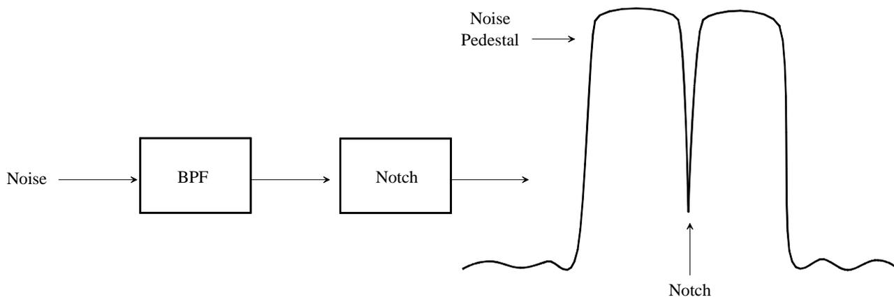
Figure 12. An NPR test generator consists of a white noise source connected in cascade with a bandpass filter and a notch filter. Notch depth can be measured with a spectrum analyzer.
