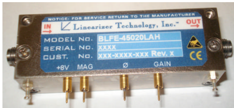
Figure 2. Q-band linearizer operating from 43.5 to 45.5 GHz.
