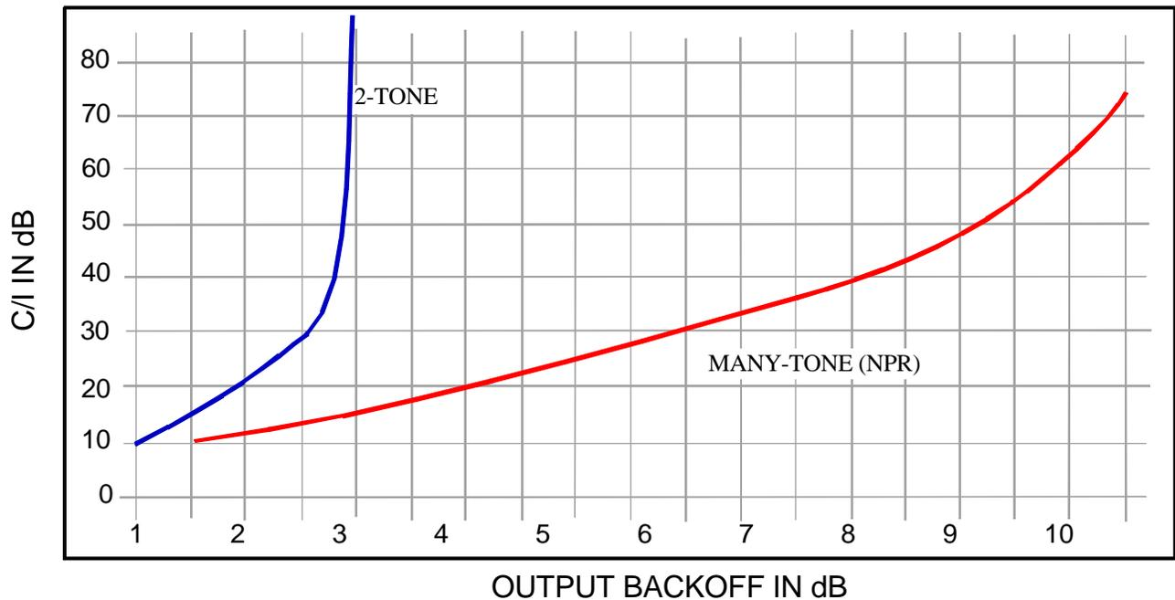
**Figure 11. C/I of an ideal transfer characteristic for 2 and an infinite number of carriers.**
