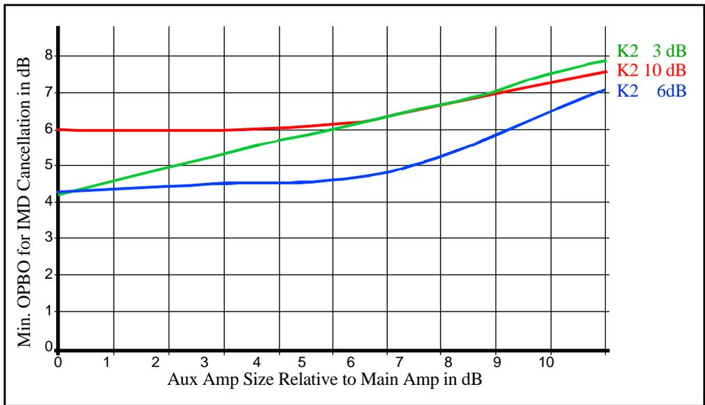
**Figure 4. The minimum OPBO for cancellation of IMD by a feed-forward amplifier depends on auxiliary amplifier size and output coupler coefficient.**
