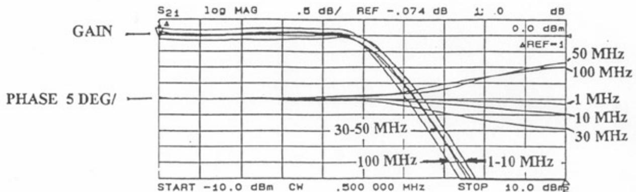
**Figure 17. Two-Tone gain and phase transfer response of C-Band SSPA.**
