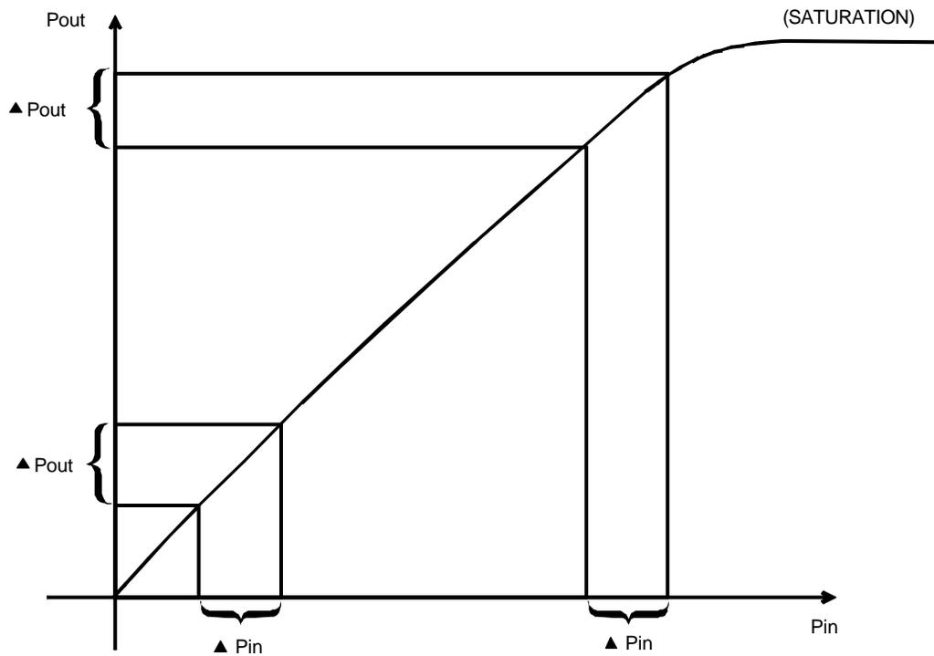
**Figure 2. Saturated output power is approached exponentially by a typical Class A SSPA.**
