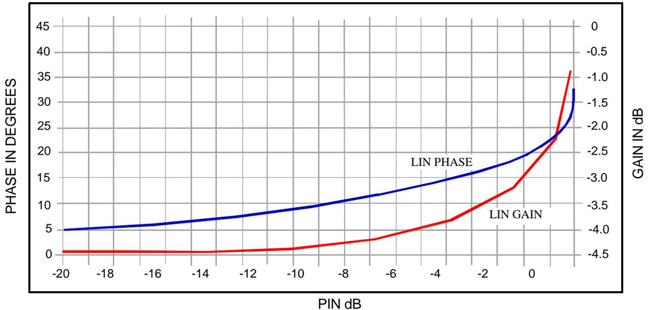
**Figure 10. An ideal linearizer response requires the rate of gain and phase change to become infinite as SAT is approached.**
