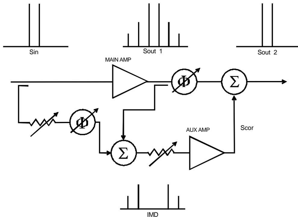
**Figure 3. Feed-forward linearization employs two loops for the cancellation of IMD.**
