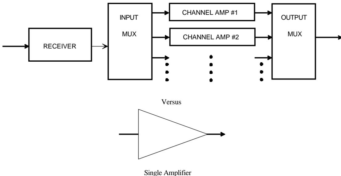
**Figure 1. In cellular telephony transmitting several carriers through a common amplifier is more cost effective than using multiple amplifiers.**
