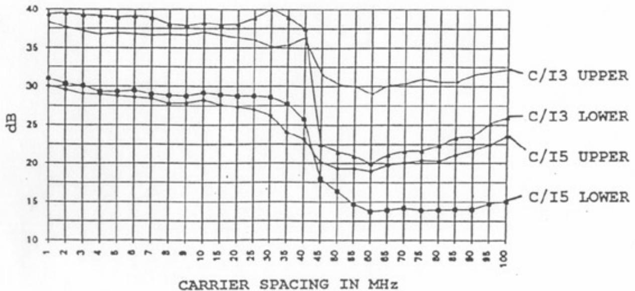
Figure 16. The linearity of SSPAs can degrade with increased carrier spacing
