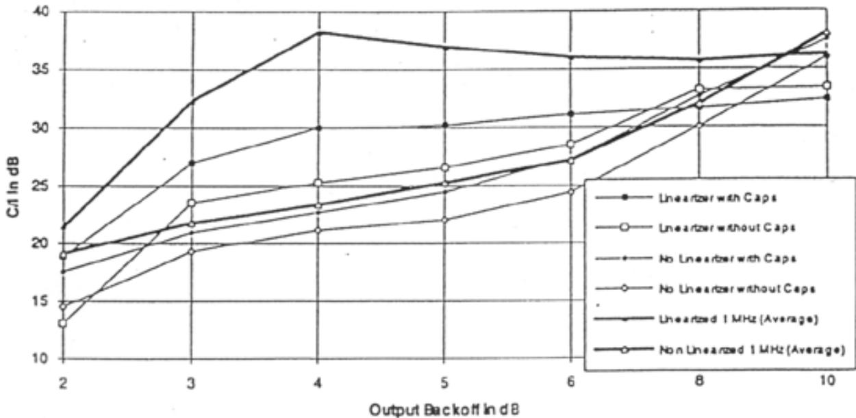
Figure 18. Improvement in C/I resulting from added drain capacitors.
