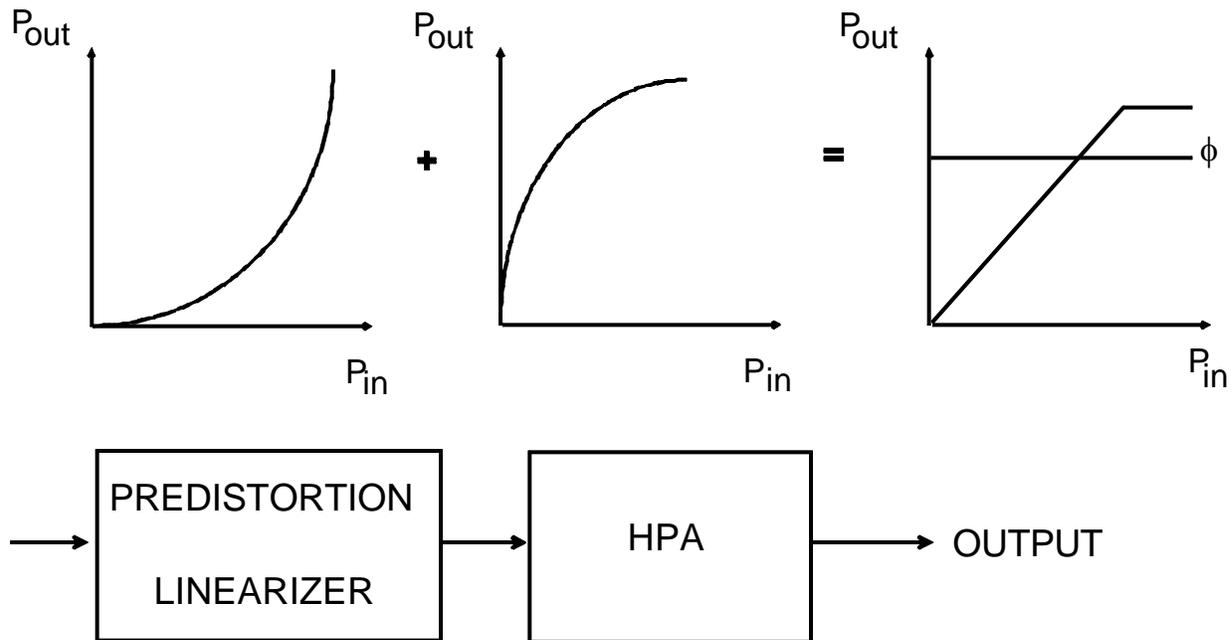
**Figure 9. Ideally the gain and phase of a linearized amplifier should remain constant up to saturation.**
