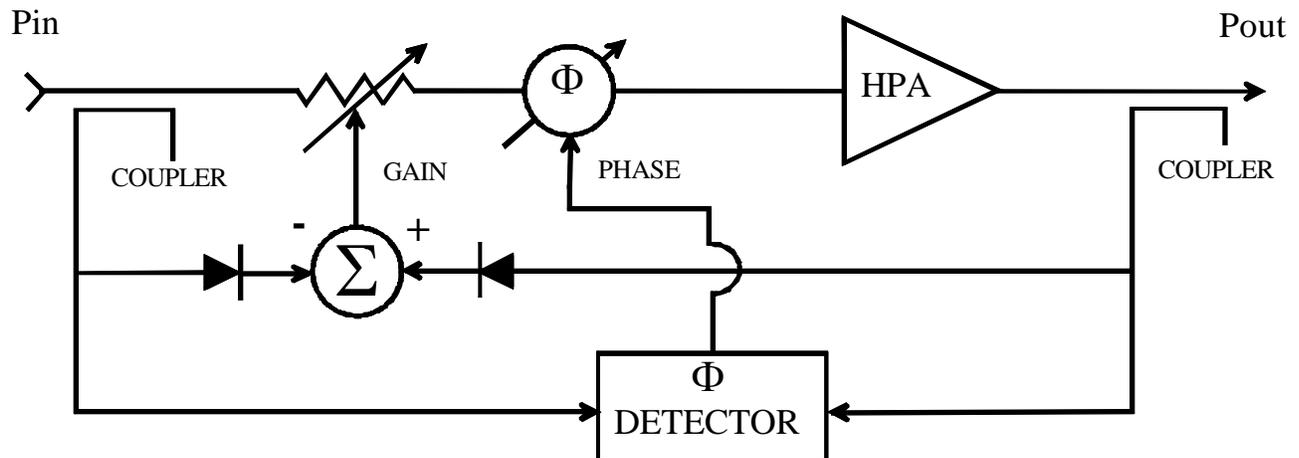
**Figure 6. The difference in magnitude and phase between input and output signals is detected and the error signals used to control amplifier gain and phase.**
