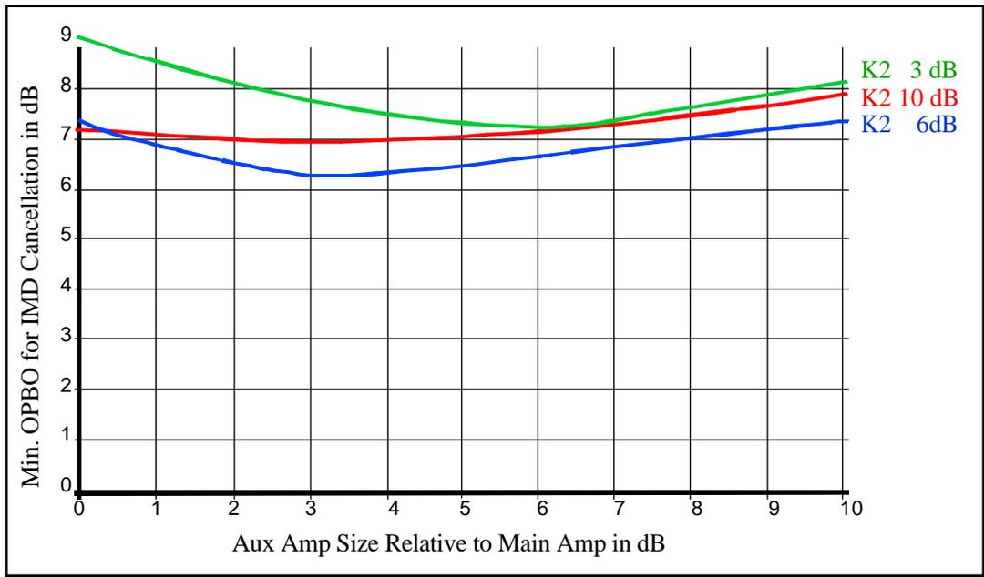
**Figure 5. Additional OPBO is required for cancellation of IMD when the output power of the auxiliary amplifier and the main amplifier are used as the reference.**
