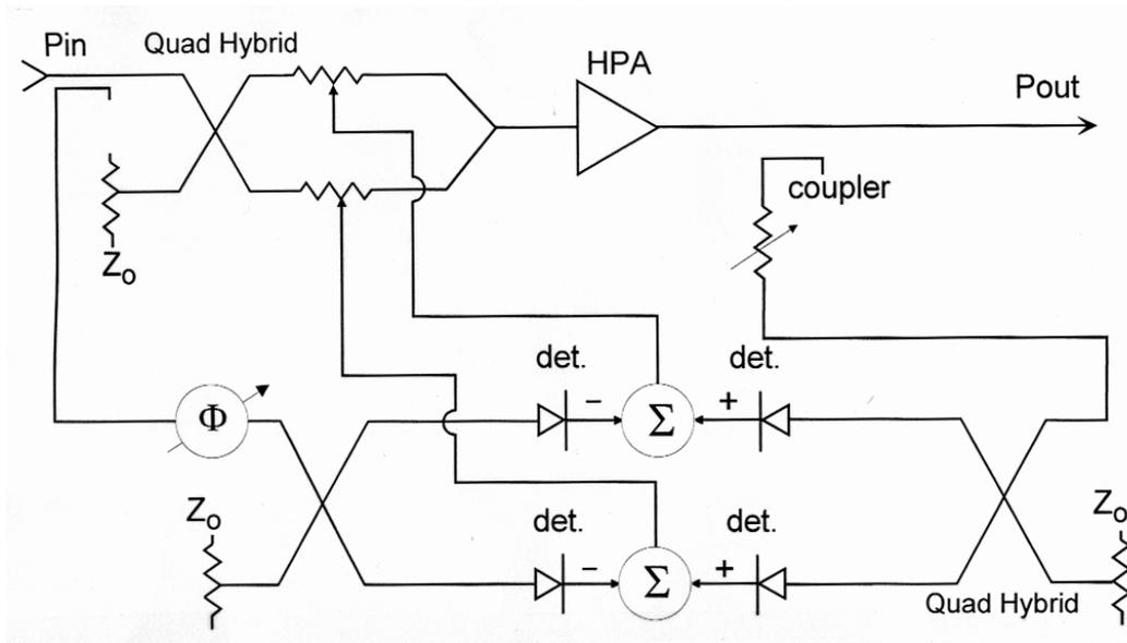
**Figure 7. Cartesian feedback eliminated the need for phase correction by using the difference between in-phase and quadrature signals to control attenuators in a vector modulator.**
