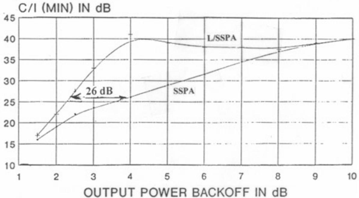
**Figure 15. C/I vs. OPBO of a Class AB SSPA and linearized SSPA.**
