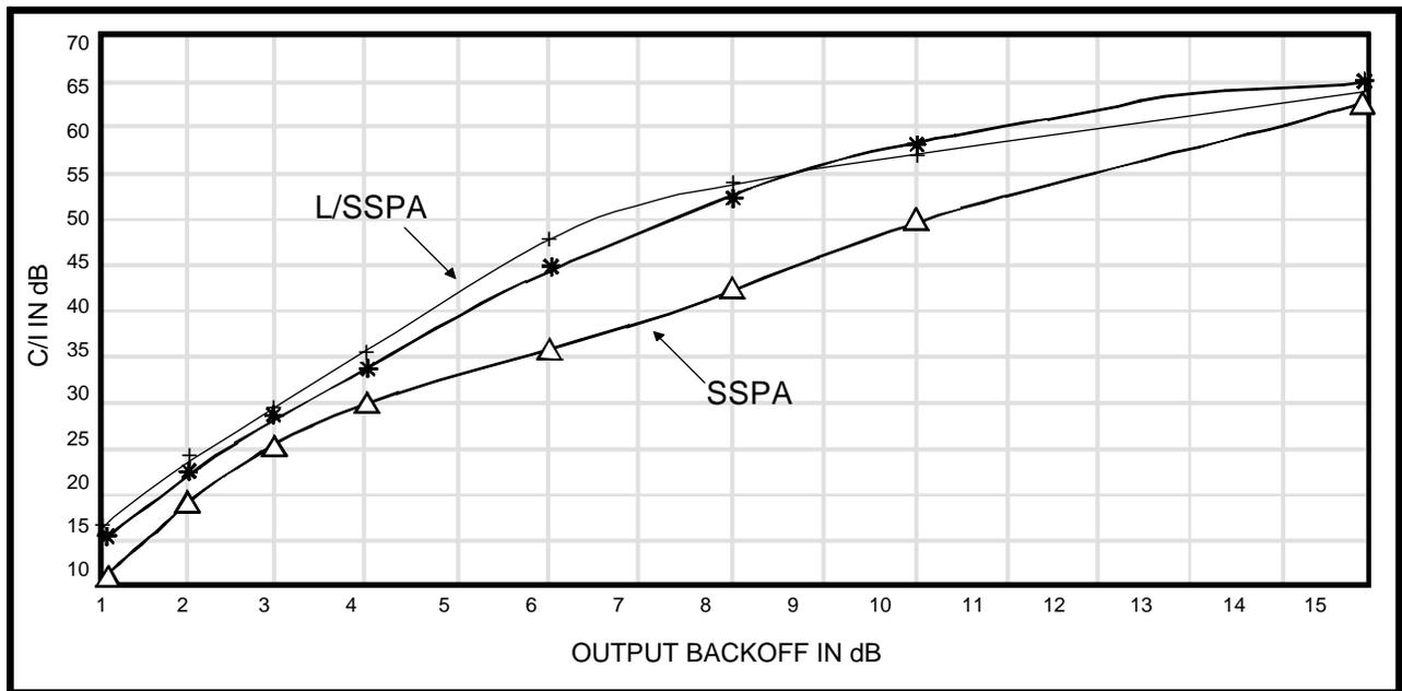
Figure 14. C/I vs. OPBO of a Class A SSPA and linearized SSPA.
