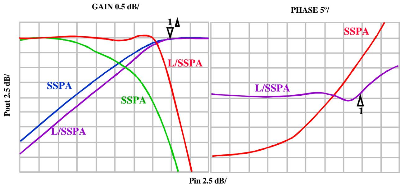
Figure 13. Transfer characteristics of a Class AB MESFET SSPA and linearized SSPA.
