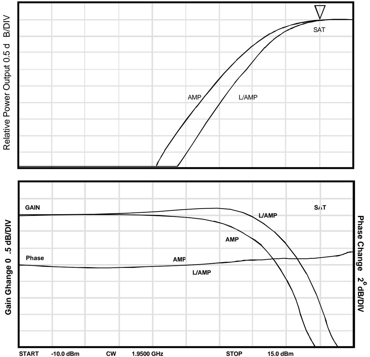
**Figure 12. Transfer characteristics of a Class A MESFET SSPA and linearized SSPA.**
