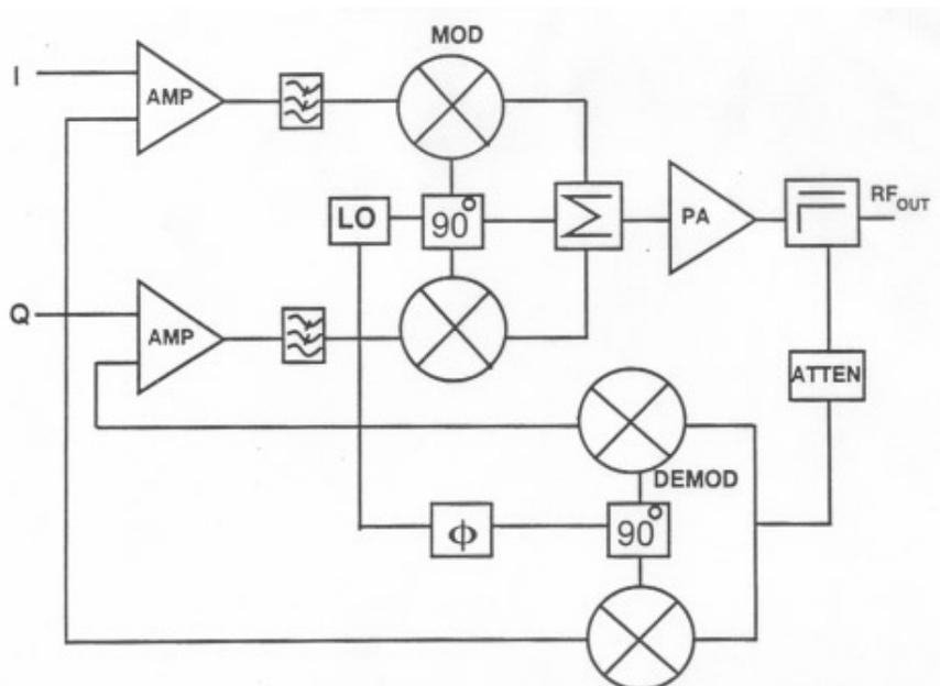
**Figure 8. Cartesian feedback is used with QPSK modulation to directly correct the in-phase and quadrature modulation signals.**
