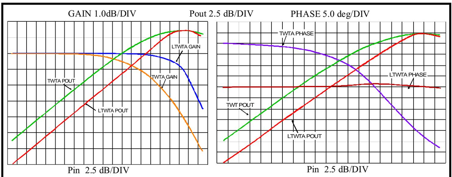
**Figure 1.** Linearizers work by correcting a TWTA's gain and phase characteristics. The 1 dB compression point is moved from about 7 dB from saturation to near saturation. Small signal linearized and nonlinearized gain are shown equal for purposes of comparison.
